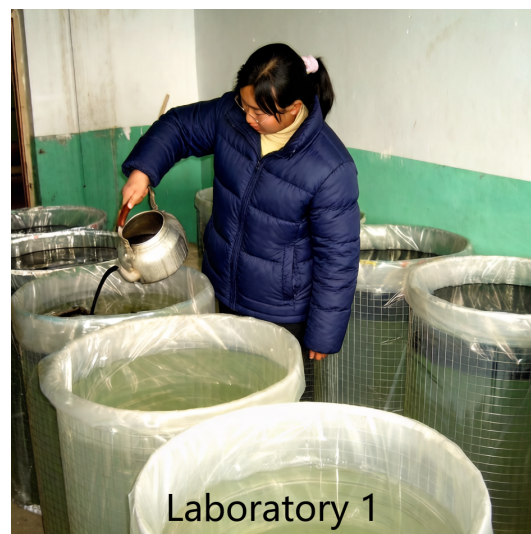
Figure 1. Laboratory 1: Divided into three groups, each containing 11 ponds. Salinity levels were 1‰, 5‰, 10‰, 15‰, 20‰, 25‰, 30‰, 35‰, 40‰, and 50‰. Freshwater was added to each group at depths of 0.5 cm, 1.0 cm, and 2.0 cm, respectively.
