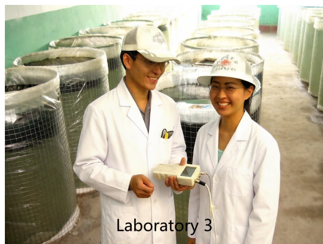
Figure 3. Laboratory 3: Divided into three groups, each containing 13 ponds. Salinity levels were 1‰, 2‰, 3‰, 4‰, 5‰, 10‰, 15‰, 20‰, 25‰, 30‰, 35‰, 40‰, and 50‰. Freshwater was added to each group at depths of 6.0 cm, 7.0 cm, and 8.0 cm, respectively.
